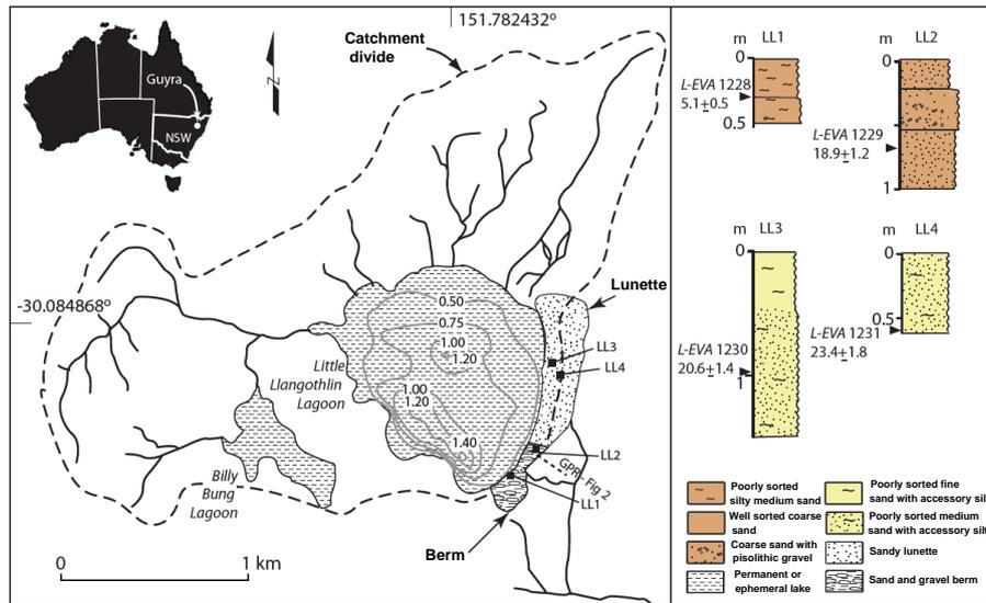
**Figure 1.** Geomorphology and sediments at Little Llangothlin Lagoon ( $30^{\circ}5'9''$  S,  $151^{\circ}46'53''$  E), 18 km NE of Guyra, NSW, showing the locations of GPR transects, sediment cores (right), and the position of OSL samples.
