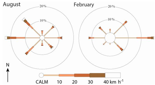
**Figure 4.** Rose of 09:00 wind direction vs. wind speed in  $\text{km h}^{-1}$  at Guyra Hospital, 1332 m a.m.s.l. (Bureau of Meteorology, 2014). Only winds above  $\sim 22$  kph are sand-carrying (based on the 12-knot threshold of Fryberger, 1979). Sand drift potential is much stronger in winter (August) than it is in summer (February) because the relationship is a power function of the wind speed and frequency of very strong winds is much lower in summer.
